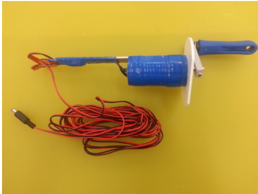
Type 1 Generator: Hand Held Hand Generator
