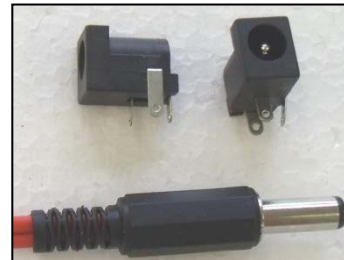
Switch the plugs to change the polarity and turning direction of handle
