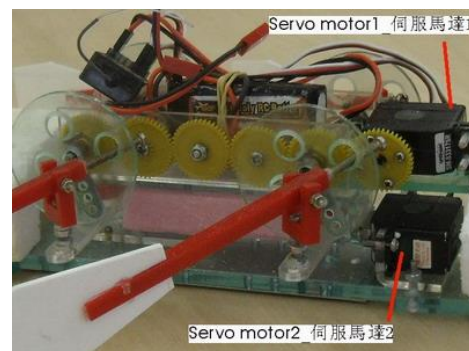
Servo motor 2: for left or right turns
