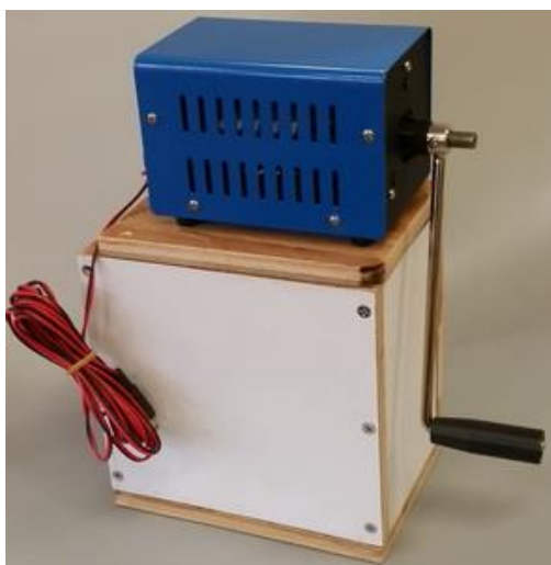
Type 2 Generator: Desktop Hand Generator
