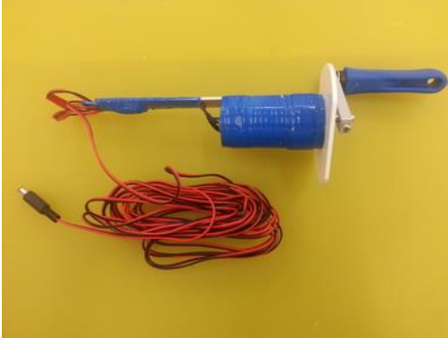
Type 1 Generator: Hand Held Hand Generator
