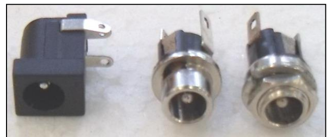
Different types of 2.1mm socket
